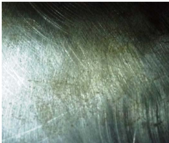
Figure 15. A photograph of an aluminium surface that was prepared by the scuff-sand and solvent clean method.
